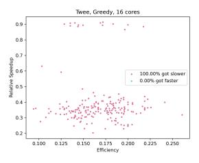
Figure 12: While the efficiency turned out to be an excellent indicator for whether a test got faster or not for the *compiler testing* benchmark, the same can not be said for *twee*. Using 16 cores and the greedy algorithm, all tests got slower and there was quite a spread of efficiencies. The overall efficiency appears to be much lower, but there is still nothing to be gained by additional cores.
