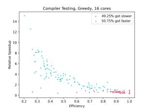
Figure 9: This figure illustrates that the closer the efficiency is to one, the higher the probability that the test will get slower when shrinking. It also appears that the relative speedup is higher the lower the efficiency.
