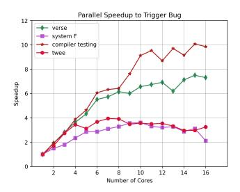
Figure 6: The acquired speedup relative to the sequential execution time when searching for a planted bug.
