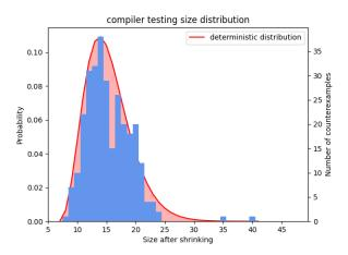
Figure 16: The measured sizes are rendered as a histogram, together with a model that represents the distribution from which they were drawn.
